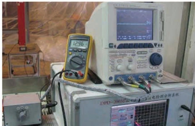
Partial discharge measurement
